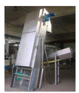
The cleaning system is made of a rake with a collecting perforated spoon capable of removing the captured particles conveying them toward the outlet. A wiper will completely remove the solids from the spoon. The cleaning system is operated by 2 roller chains driven by a single gearmotor.
