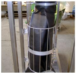
After a few hours it is possble to reach a 20% dry solids with a reduction in volume of about 10 times. The bags, closed with a special twisting tool, optional, are removed and deposited in a suitable area for a further reduction in volume due to evaporation.
