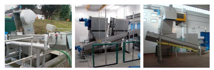
Materials of construction for fabricated parts: \*Stainless Steel AISI304 / \*Stainless Steel AISI316
