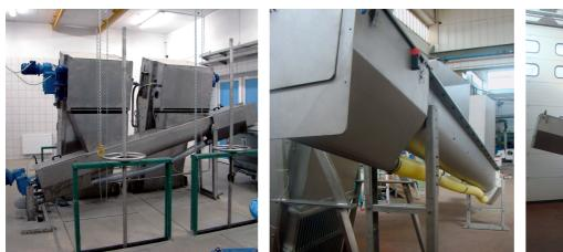
Here a cylindrical sieve allows the material conveyed to be permanently relieved of any remaining liquids. In front of the outlet of the compacting and draining module there is a cover fixed on the top that opens only when sufficient dewatered waste material has accumulated inside the sieve until forming a real plug.
