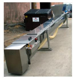
The following part is the transport zone, where the screenings free of organic matter are conveyed; at the end of the transport module the drain module completely eliminates the liquid residues coming from the washing zone, repeating the waste washing a second time.
